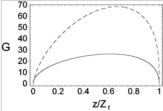
Comparison of the instability gain G plotted as a function of axial distance for ion beam with velocity tilt (solid curve) and without velocity tilt (dashed curve).
