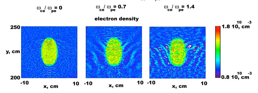
In the presence of a solenoidal magnetic field, whistler waves are excited, which propagate at an angle with the beam velocity and can perturb the plasma ahead of the beam pulse.
