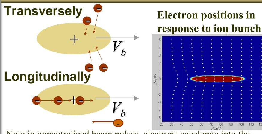
Note in unneutralized beam pulses, electrons accelerate into the beam attracted by space potential: indicating the inductive field is important even for slow beams!
