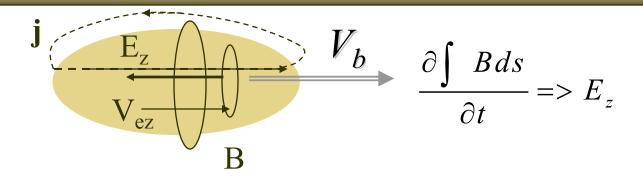
Alternating magnetic flux generates inductive electric field, which accelerates electrons along the beam propagation\*. For long beams canonical momentum is conserved\*\*  $mV_{ez} = \frac{e}{c}A_z$
