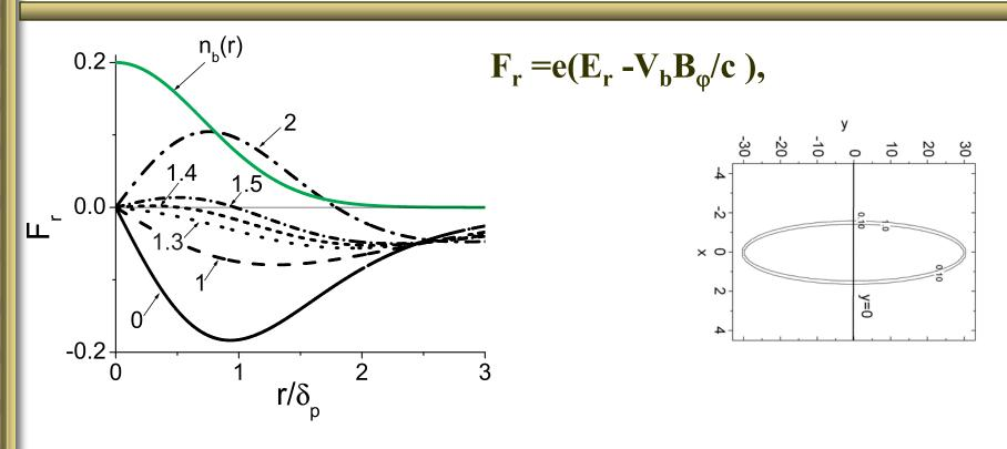
Normalized radial force acting on beam ions in plasma for different values of  $(\omega_{\rm ce}/\omega_{\rm pe}\beta_{\rm b})^2$ . The green line shows a gaussian density profile.  $r_b = 1.5\delta_{\rm p}$ ;  $\delta_{\rm p} = c/\omega_{\rm pe}$ .
