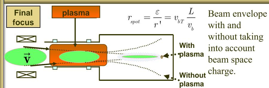
with and without taking into account beam space charge.
