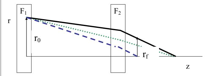
$r_{sp} \sim r_f 2\Delta v_b/v_b$  chromatic effects in the final focusing element
