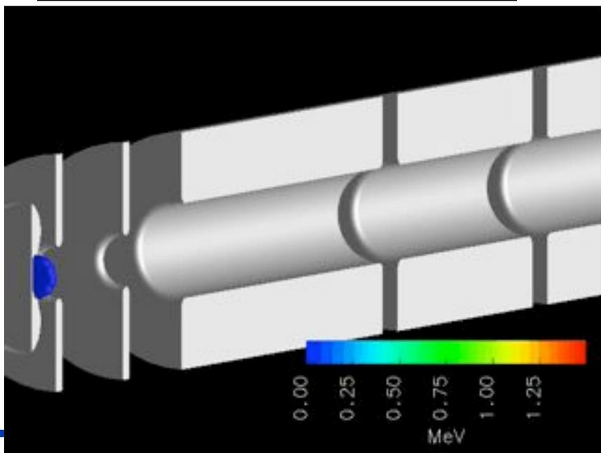
Video: Warp 3D simulation of NDCX-II, including random offsets of solenoid ends by up to 1 mm (0.5 mm is nominal)
