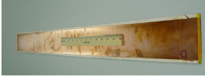
A one-meter long stripline of the castable dielectric. This line has a relative dielectric constant of about 40 and is relatively flexible.
